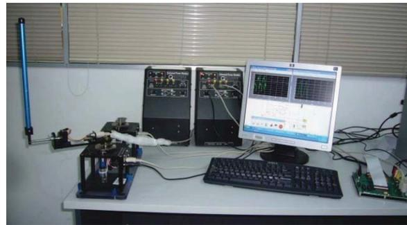
Figure 1. Inverted pendulum and controller.
