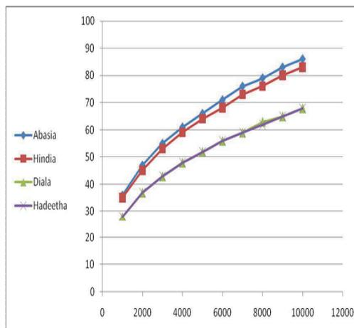
Figure (1) The Relation Between Flow Rate (Q) in gpm and Pipeline Diameter in inch For Supplying Water to Basra City from Dams
