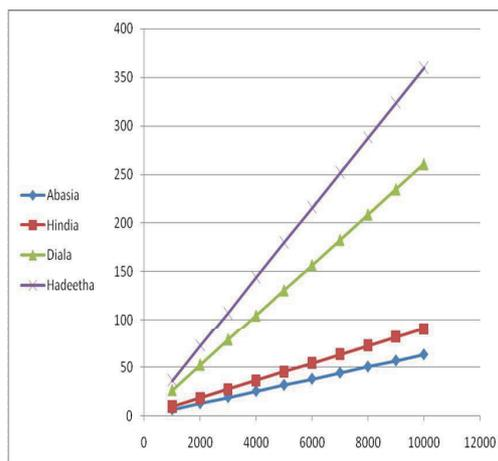
Figure (2) The Relation Between Flow Rate (Q) in gpm and The Hydroelectric Generated power in KW From Supplying Water to Basra City from Dams
